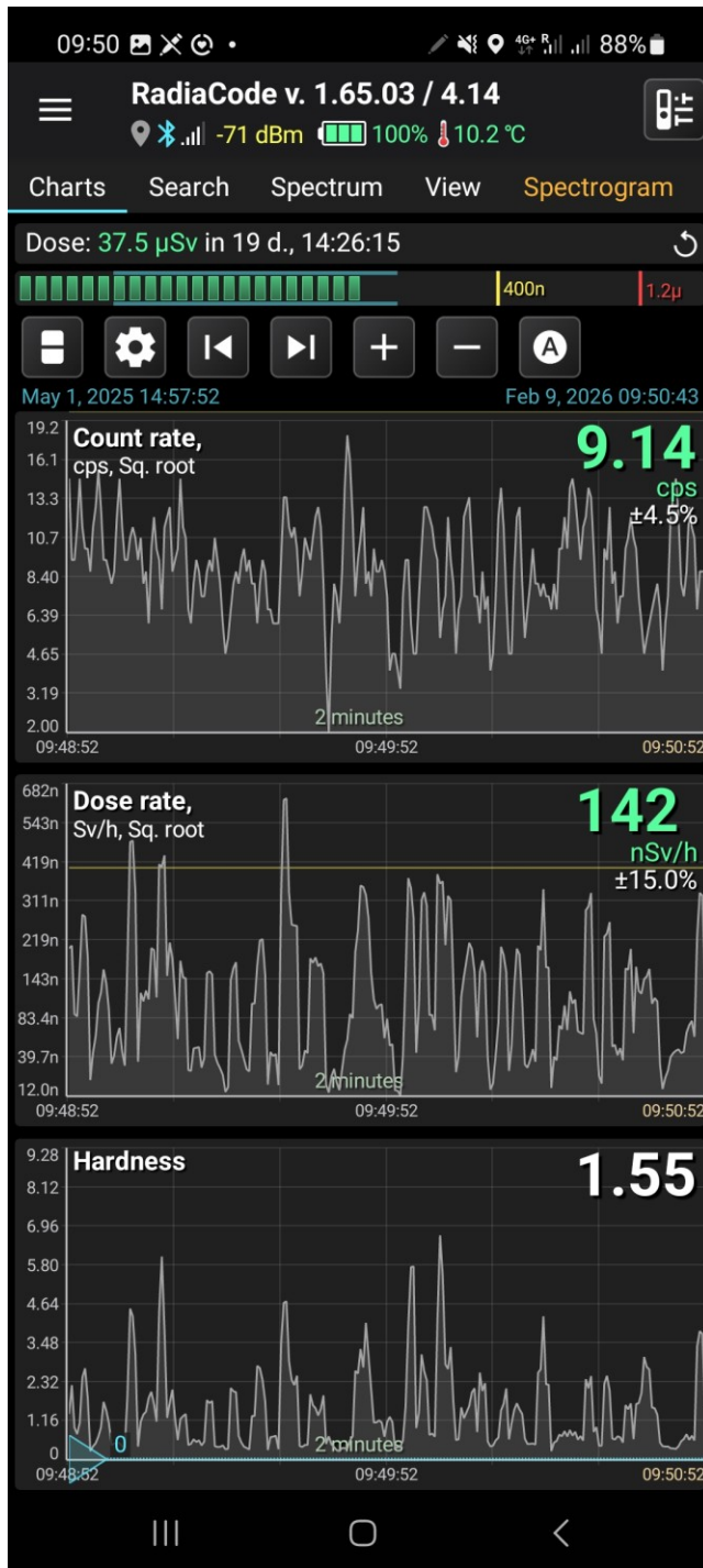
Figure 6 - Two-minute time series from Experiment 2 showing count rate, dose rate and hardness
