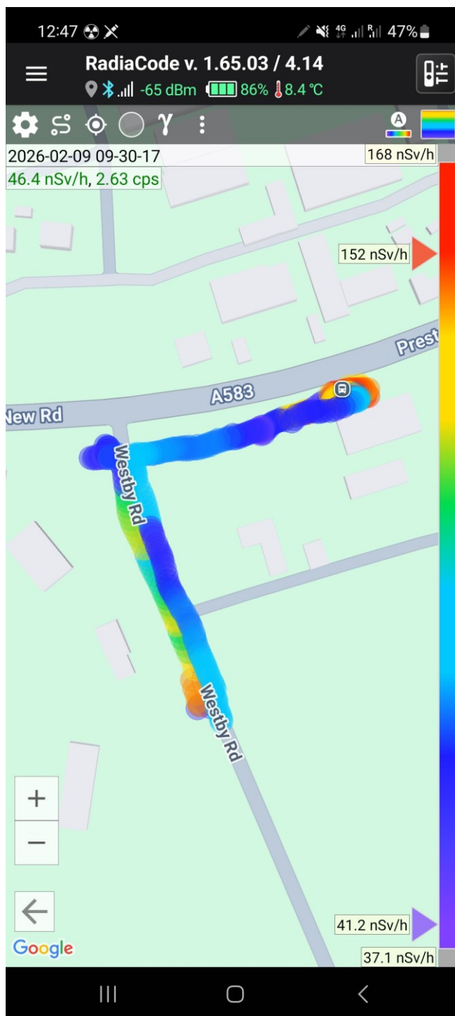
Figure B2 presents the corresponding count rate track over the same route and time window. Spatial patterns are broadly consistent with the dose rate distribution.
