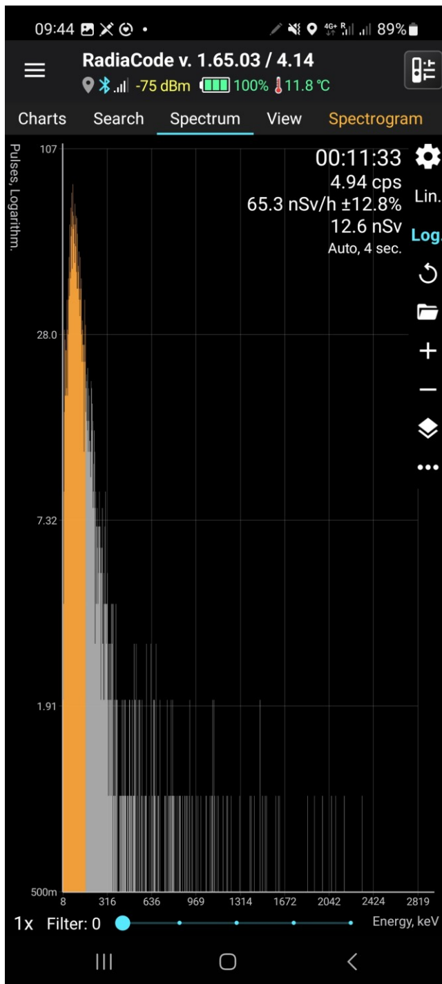
Figure 3 - Gamma energy spectrum from Experiment 1 acquired over an approximately 10-minute accumulation period (00:11:33; mean 4.94 CPS; 65.3 nSv/h).
