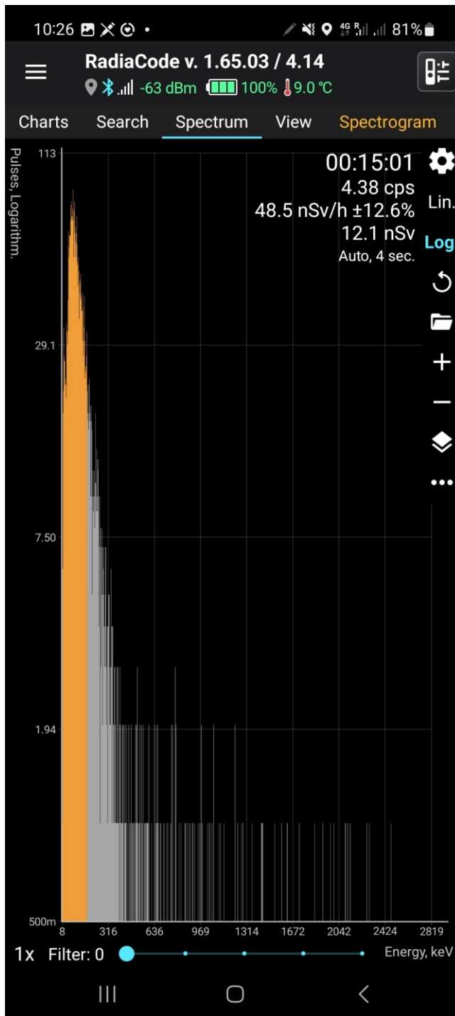
Figure 13 – Gamma energy spectrum accumulated over fifteen minutes at the westward control location.
